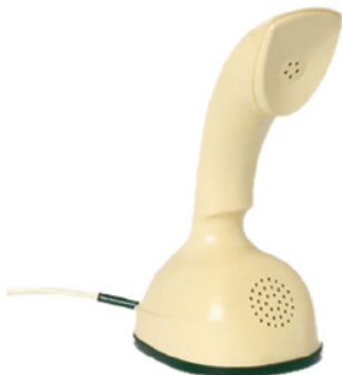
Figure 1.3 Telephone housing made of Bakelite [Image source: Deutsches Kunststoffmuseum (German Plastics Museum)]
