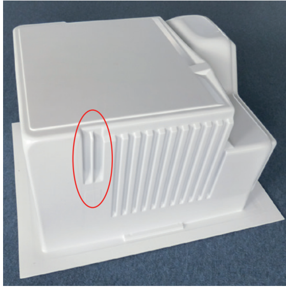
Figure 2.12 Refrigerator interior tray in impact-resistant polystyrene, positively formed. Detail of chill mark, see Figure 2.13 and Figure 2.14
