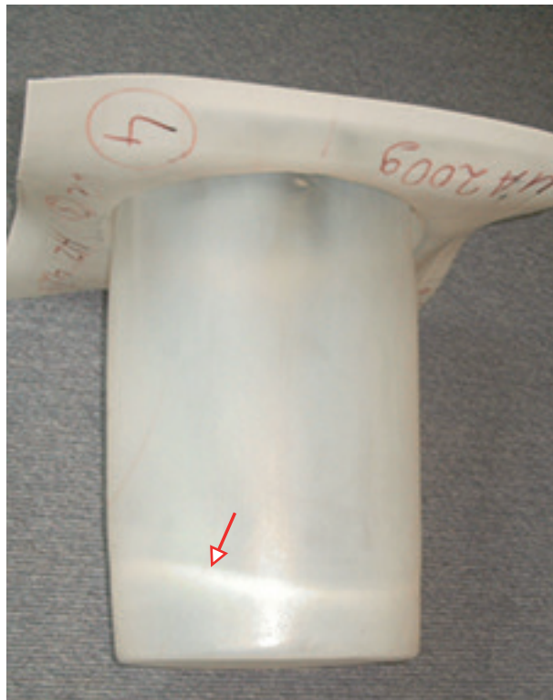
Figure 2.17 Negatively formed part in PEHD with chill mark caused by the plug-assist tool
