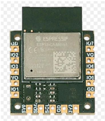
Abb. 2.6: ESP32-Board – CodeCell (Quelle Microbots)
