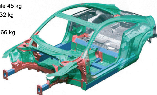
Abb. 3.19: Audi TT in Multi-Material-Design (Quelle: Audi 2006)
