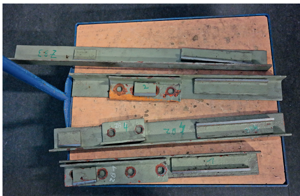
Fig. 1: Structural members of a power tower in as-received condition Angle iron 60 \times 40 \times 5,5 .
