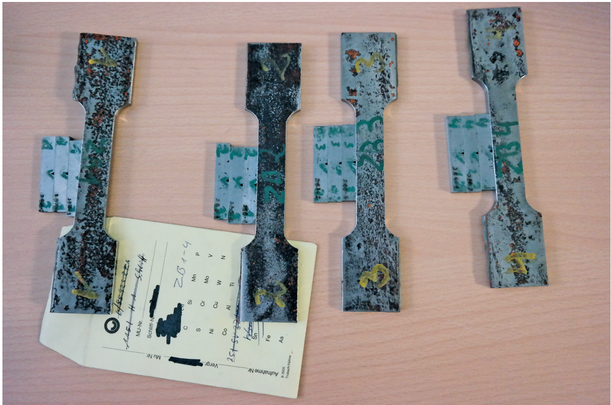
Fig. 3: Tensile and Charpy V-notch impact testing specimens ZB1 (left) to ZB4 (right) machined in longitudinal direction from the structural members.
