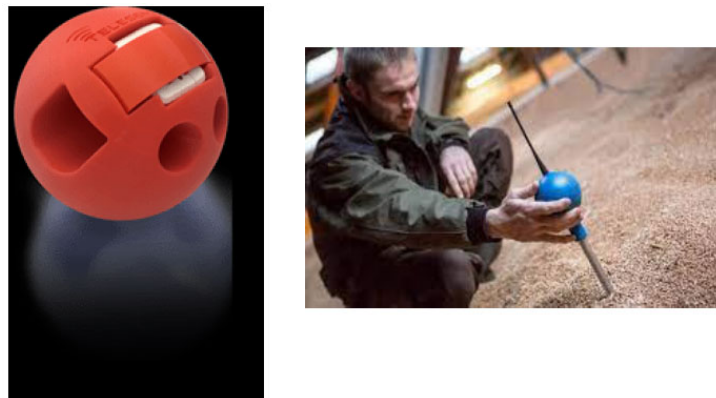
Fig. (2). GrainSage by Telesense to keep grain fresh (Courtesy: https://www.futurefarming.com/smart-farming ).
