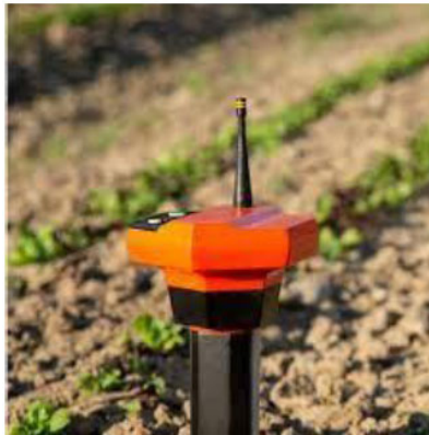
Fig. (5). Teralytic: Wireless NPK sensor for monitoring soil health (Coutesy: https://www.producer.com/crops/independent-probes-take-the-measure-of-the-soil/ ).
