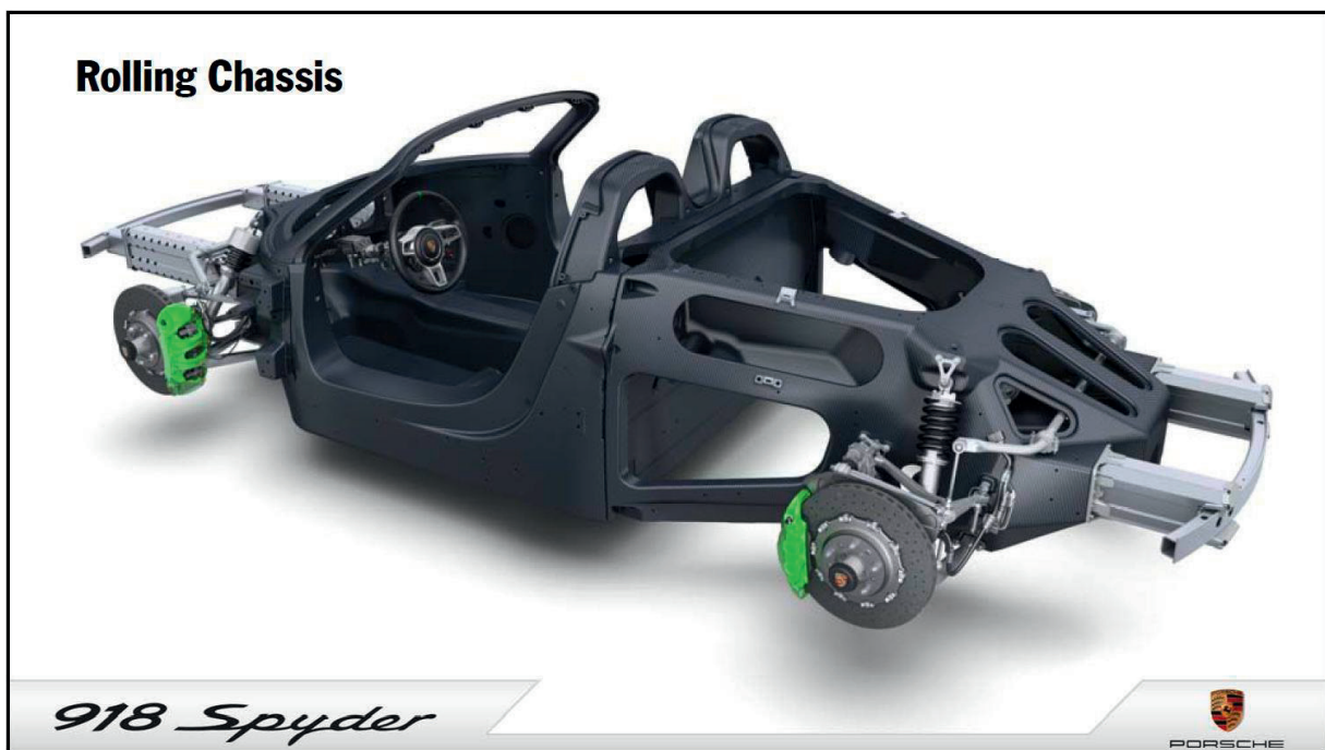
Figure 2.1.1: Rolling chassis of the Porsche 918 Spyder [2.1.6]
