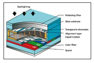
of glass, electrode, alignment layer, liquid crystals, alignment layer, electrode, sheet of glass, polarizing filter. Between the substrates are the thin film transistors and color filter panels, which provides the red, green, and blue primary colors, and the liquid crystal layer. The screen is illuminated from behind using fluorescent backlight.
