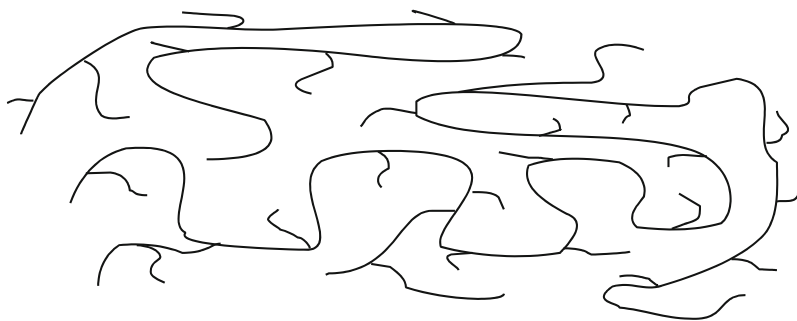
Figure 3.2 Representation of a branched polymer
